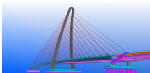
Figure 3: Elements and assemblies of the projected bridge
